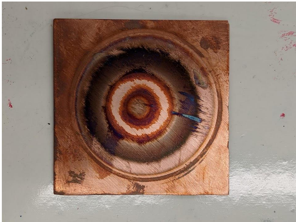
Picture 2: Oxidation on copper plate after a deposition
